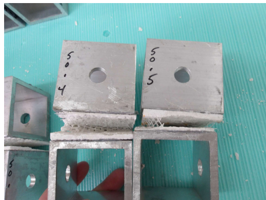
PhotoNo. 12 ASTM C297 – Representative Post-50 Cycle Freeze/Thaw Exposure Cohesive Failure Mode
