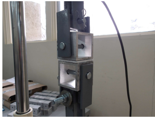
PhotoNo. 10 ASTM C297 – Load Application Fixturing Detail
