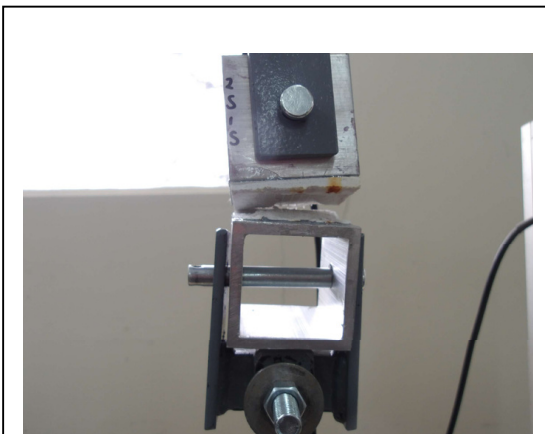
PhotoNo. 11 ASTM C297 – Representative Post-25 Cycle Freeze/Thaw Exposure Cohesive Failure Mode
