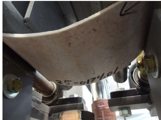
PhotoNo.8 ASTM C880 – Representative Specimen Failure Mode: Lengthwise Orientation (Wet Condition)
