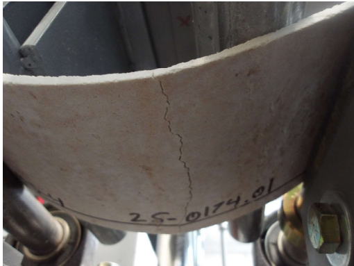
PhotoNo.7 ASTM C880 – Representative Specimen Failure Mode: Widthwise Orientation (Dry Condition)
