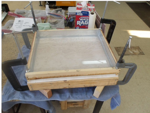
PhotoNo.3 ASTM C1185 Water Penetration Evaluation–Test Setup
