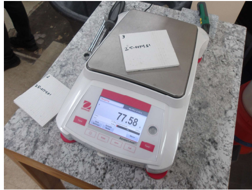
PhotoNo.2 ASTM C97 – Absorption & Density Test (Dry Mass Determination Stage Depicted)
